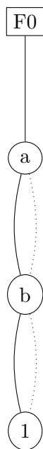
Figure 7: The function f(a,b) = (a = b) as a BDD with complement edges as generated by CUDD
